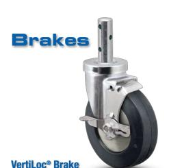
A popular side-operated brake that employs cam action to lock brake pad across entire surface of wheel tread. Brake locks wheel only, and the swivel radius of the caster is not affected by this brake design. All steel construction provides positive, reliable braking under a variety of operating conditions and wheel tread types.
